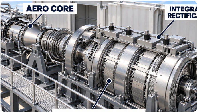
CONCEPT Aero core driving Hyper Tech generators with integrated rectification: 800 V DC leaves the generator.
